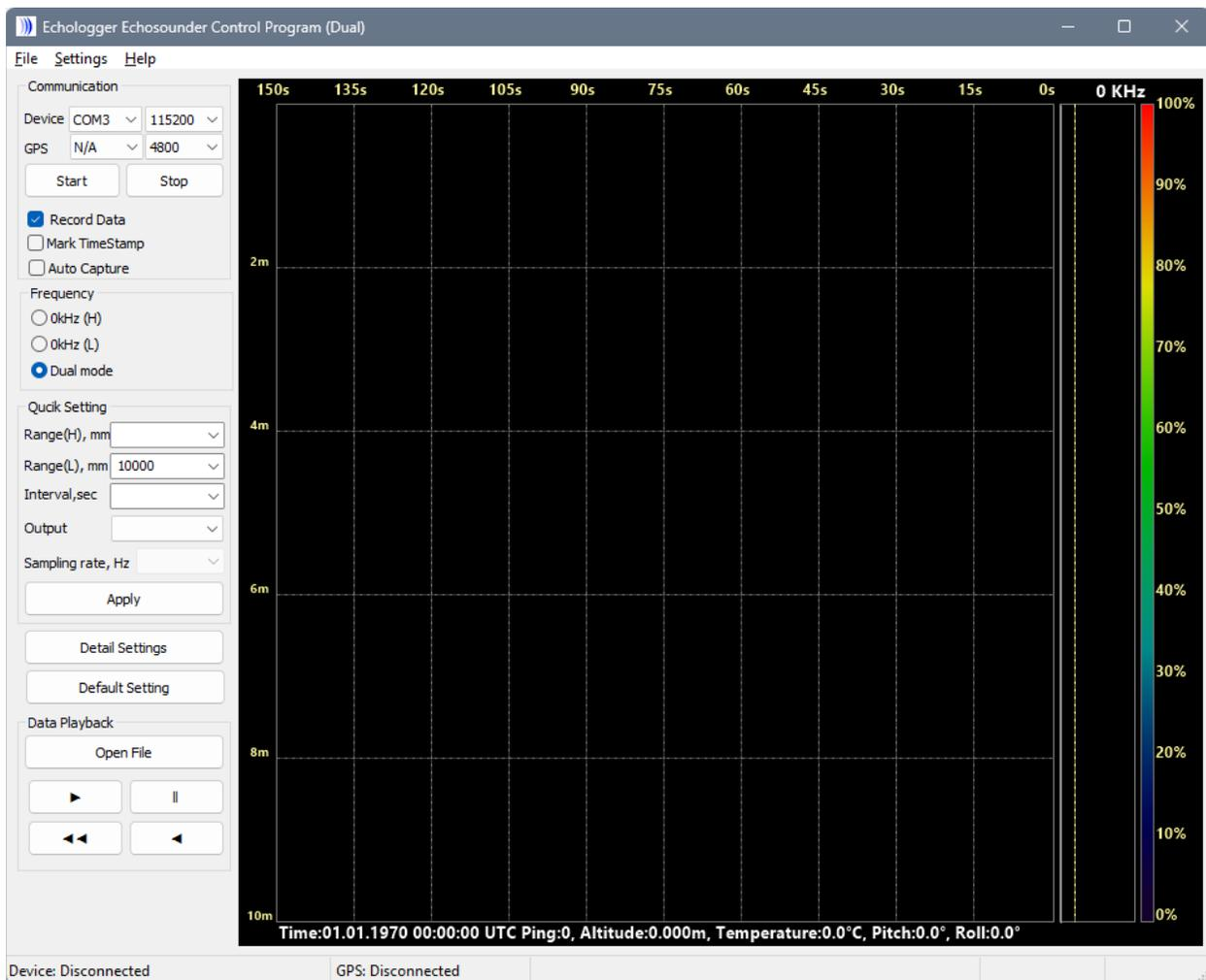
On the left-hand side of the window you can see the different parameters that can be changed. If both frequencies are to be used, ensure that the frequency option is set to “Dual mode”
