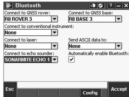
Tap Config and make sure that Bluetooth is switched on. On a TSC2 controller, make sure that the [turn on Bluetooth] and [Make this device discoverable to other devices] check boxes are selected. On a Trimble CU (model 3) controller, select the power tab and then make sure that the [enable Bluetooth] and [Discoverable] check boxes are selected. On a Trimble CU controller, make sure that the [Enable Bluetooth] checkbox is selected.
