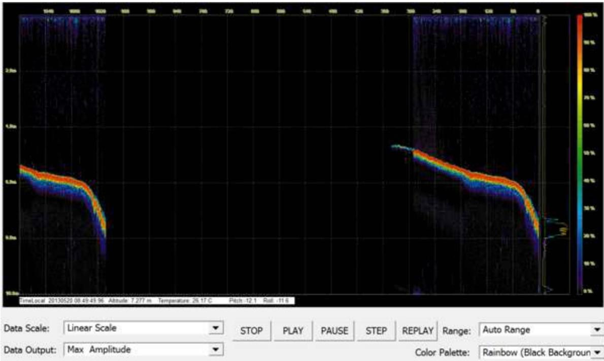
When the real time returns are being shown in the echogram, the altitude is determined when the signal passes the set threshold parameter. For this reason, Altitude threshold, Deadzone, and Gain are the important settings when tuning the system. See example below.
