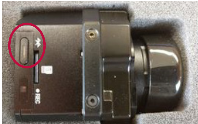
FIGURE 7. Starting the Bluetooth Connection on the Camera
