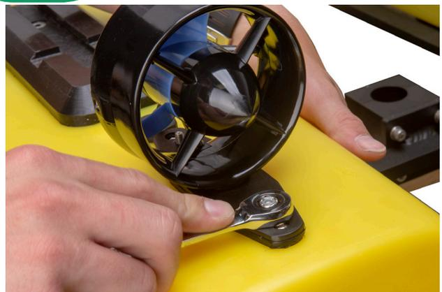
With  $\frac{3}{8}$ <sup>th</sup> socket or end wrench remove the nuts on thruster plate that are on either side of the thruster.
