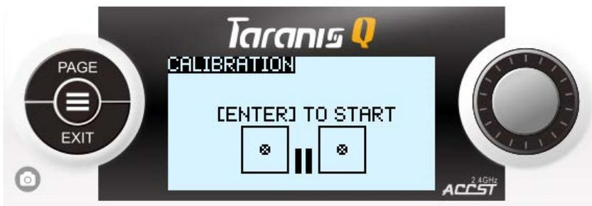
6. Move the sticks and points along each extreme top, bottom, left, and right. During this step the knobs should be turned to their extremes as well. Finally press the silver button to confirm
