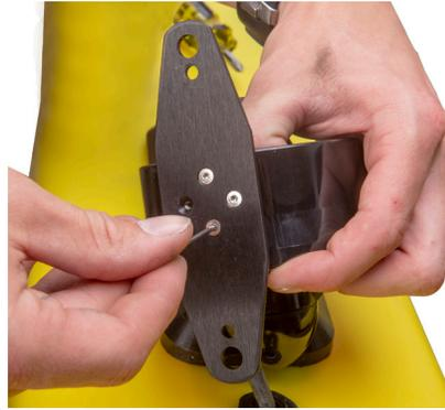
Once nuts are removed, the thruster plate and thruster will lift off the boat and expose the m3x6 allen screws that hold the thruster plate to the thruster. Remove the thruster plate from the thruster by removing those four screws with 2mm allen key. If you are replacing the thruster skip to step 10.
