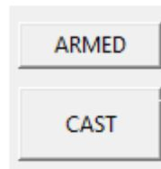
Once the cast has begun the system will again reset the “Current Depth” to zero. Next it will descend to the desired depth, pause for two seconds, and then come back up and reset “Current Depth” a third time. After this the system will disarm itself.
