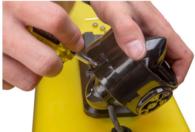
Remove the four #2 Phillips screws along the outer edge of the thruster.
