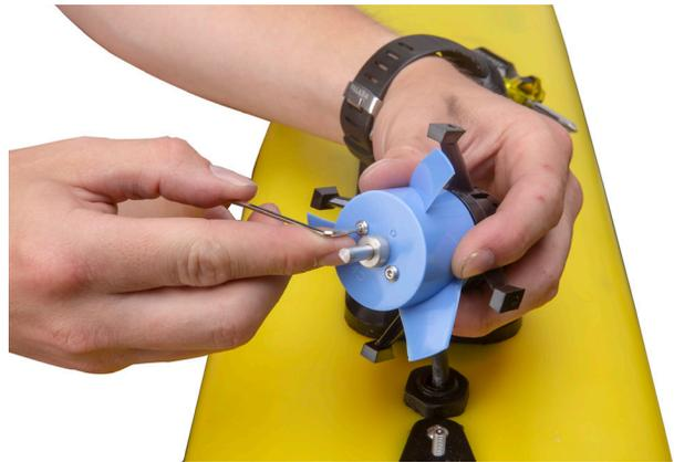
Remove the 2mm allen screw that holds the propeller to the motor assembly.
