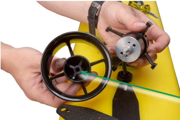
Make sure to clean inside of the nozzle and tail cone with a non-abrasive brush.
