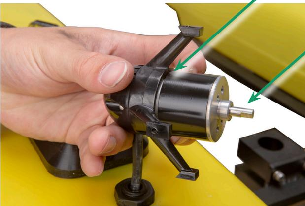
Most importantly clean the area between the motor assembly and the thruster base as well as the gap, as long grass, fishing line, anything thin and long will end up in there. A paperclip or small Allen key works for cleaning it out. Alternatively, you can remove the set screw and pull the two pieces apart for better access.
