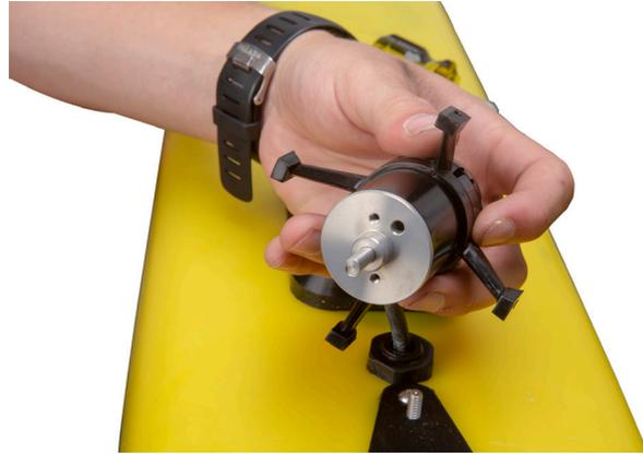
Remove the propeller from motor assembly by putting pressure on the motor shaft while pushing the propeller off of the the motor assembly. Be careful not to put too much pressure on the propeller fins. No further disassembly is required.
