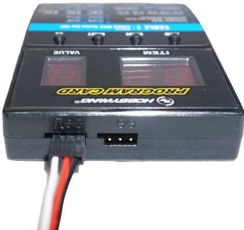
Ensure the boat has power and plug the programming card into the port on the ESC. The programming card will start up as soon as you turn the boat on.
