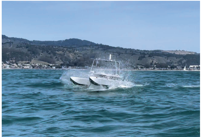
Independently articulating pontoons
