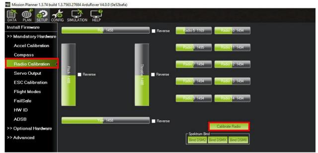
5. Two dialogue boxes will appear. The first is a warning that the boat should be unpowered, if this is not possible then make sure the ESCs that control the motors are switched off or disconnected. The second box gives directions on what to do during the calibration (see next step). Get through the boxes by clicking "OK".
