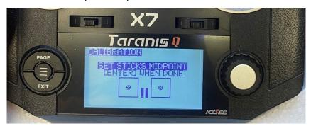
6. Move the sticks along each extreme top, bottom, left, and right. During this step the knobs should be turned to their extremes as well. Finally press the silver button to confirm
