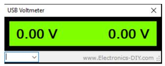
3. Navigate to "Ports (COM & LPT)" and look for a COM port labeled "USB Serial Device". Enter this number into the USB Voltmeter program in the bottom left of the box.
