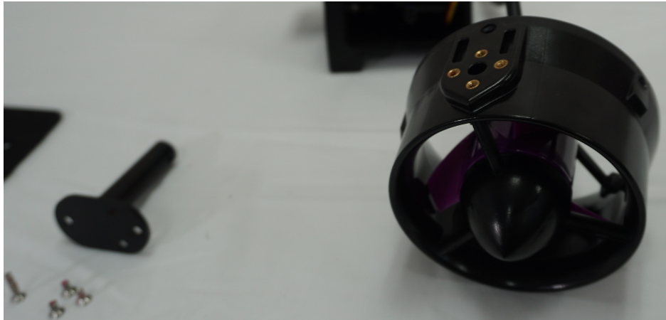
Figure 67: Thruster Adapter Shaft Removal
