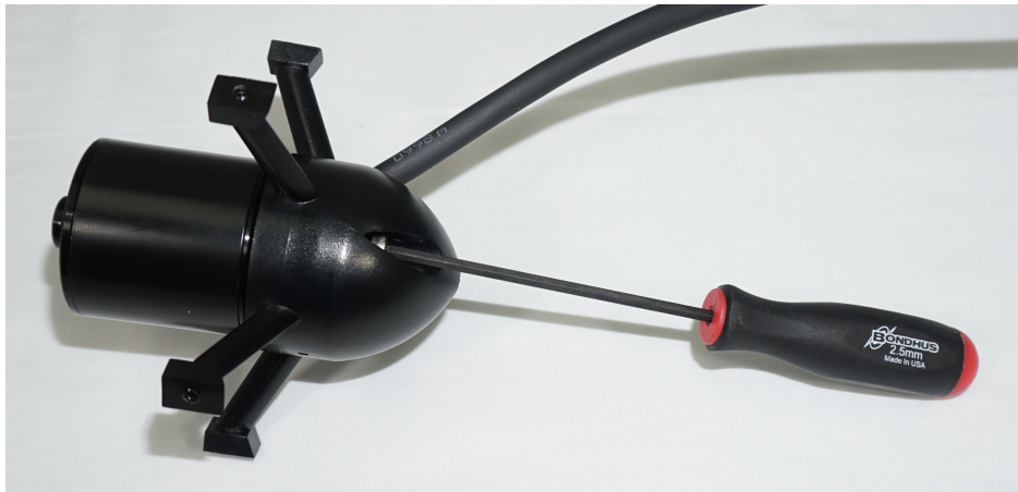
Figure 77: Motor Housing Removal
