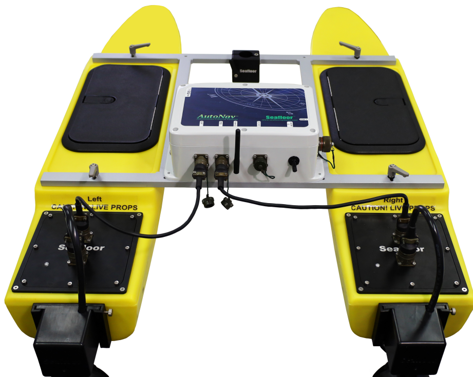
Figure 12: HyDrone™ ASV Servo Assembled
