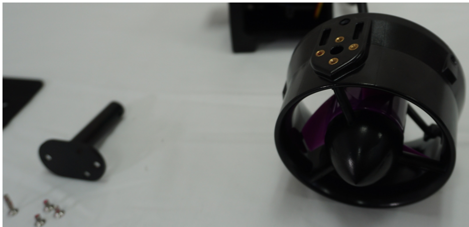
Figure 73: Thruster Adapter Shaft Removal
