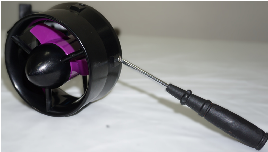
Figure 74: Thruster Housing Removal
