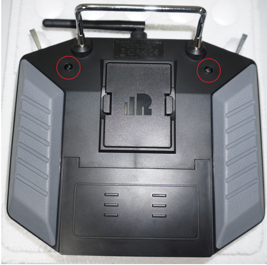
Figure 103: RCU 2x Screw Locations
