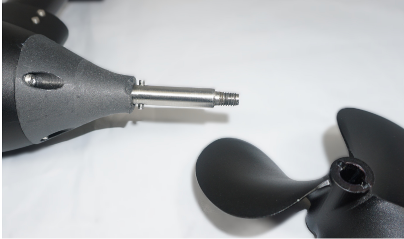
Figure 101: Prop Shaft With Alignment Pin
