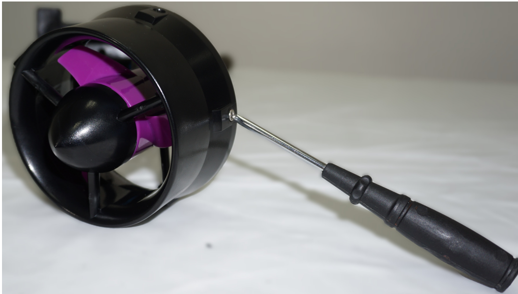
Figure 99: Thruster Housing Removal
