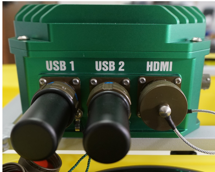
Figure 20: USB Covers Installed
