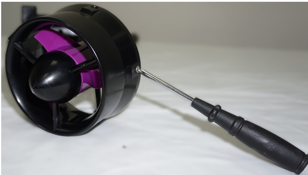
Figure 105: Thruster Housing Removal
