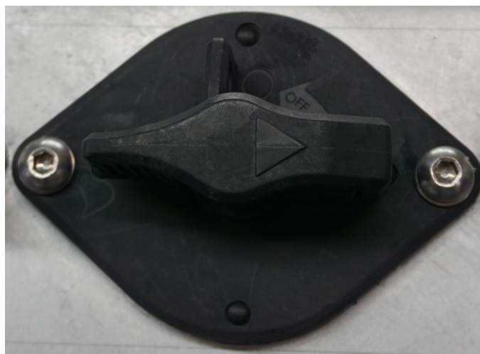
Figure 27: Pontoon Shutoff Switch - On
