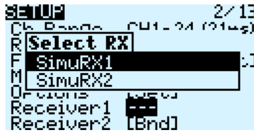
Figure 79: RCU Binding Screen - SimuRX1/2 Is Only Used For Simulation
