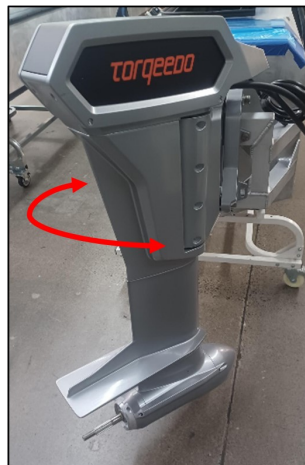
Figure 97: Hold Thruster During Purging Process
