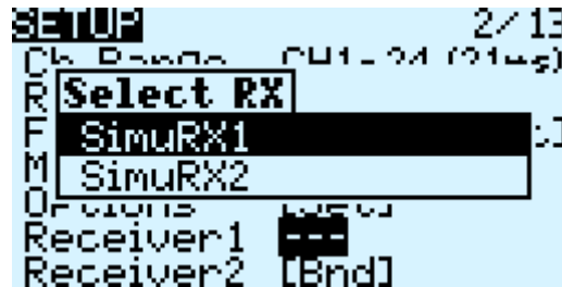
Figure 73: RCU Binding Screen - SimuRX1/2 Is Only Used For Simulation
