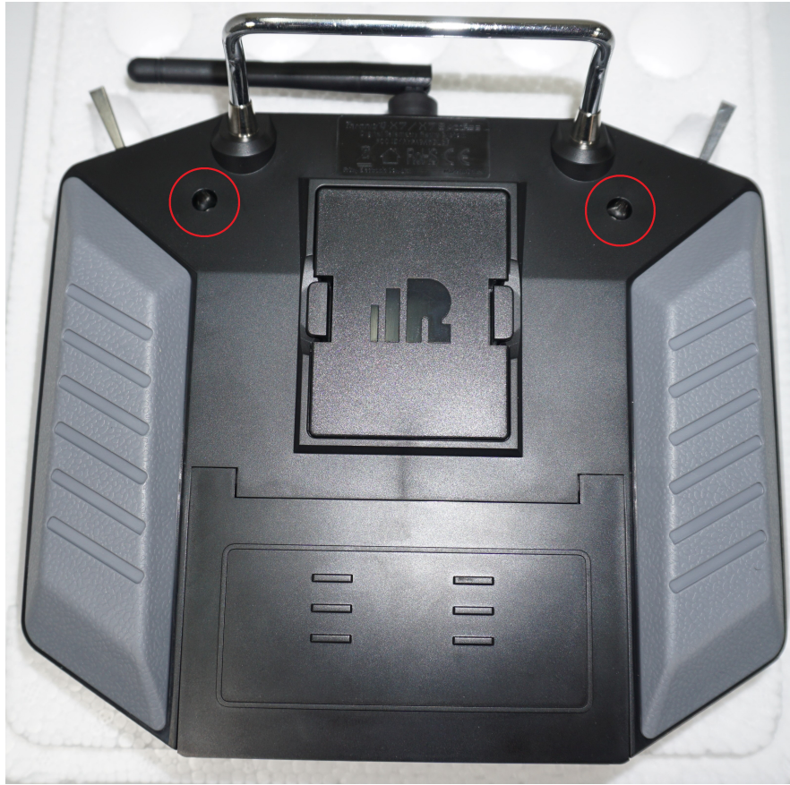
Figure 107: RCU 2x Screw Locations
