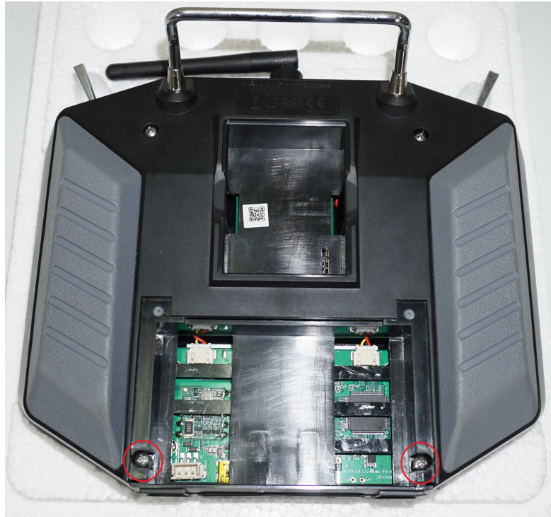
Figure 108: RCU Additional Screw Locations
