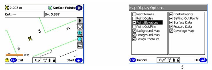
Remember that if loads of points are stored, this option can slow down the CE device and make the map hard to read, so switch of again if required.
