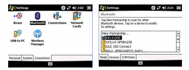
Enter the passkey (usually this is 1111) and enter the partnership settings, by checking the serial port service. After this, the Sonarmite is visible under the tab Devices.
