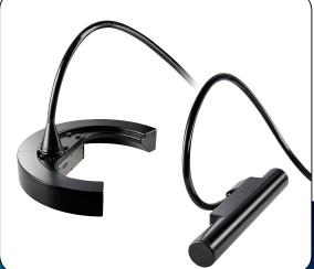
The SeaBat 7111 produces bathymetry data suitable for the generation of high resolution hydrographic charts exceeding international standards in water depths from 3 to 1000m. Operating at 100kHz, the system forms 101, 201 high-density, equi-angle or 301 equi-distant beams to cover a total receive sector of 150°.
