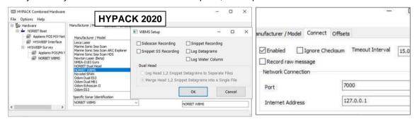
If using **HYPACK 2021**, enable the **Use Pass Through Position, Heading and MRU** option. This provides the navigation solution, simplifying the setup by removing the need for the Applanix POS/MV Network devices that were required in previous versions.
