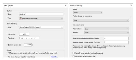
Under Raw Data Recording, for standard bathymetric data collection select the **NORBIT** System and **None** for Packet Storage, Water Column and Snippets.
