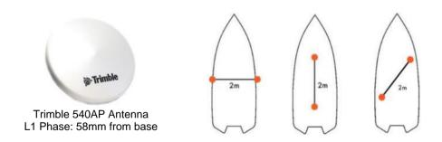
The Primary Antenna (Ant 1) should be nearest to the sonar so that offset measurement errors are minimized. The Secondary Antenna (Ant 2) should be a fixed distance from the Primary Antenna. It is recommended that the antennas be at least 2m apart for optimal performance. The antennas should be positioned parallel to the water surface to within 2-3cm.
