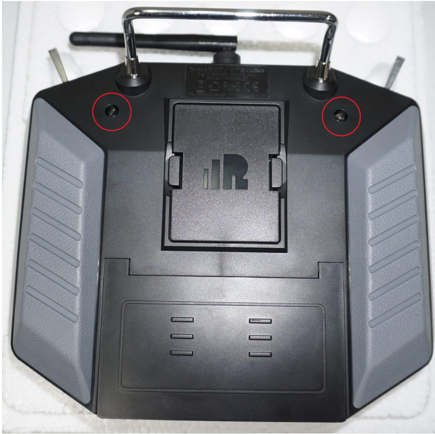
Figure 91: RCU 2x Screw Locations
