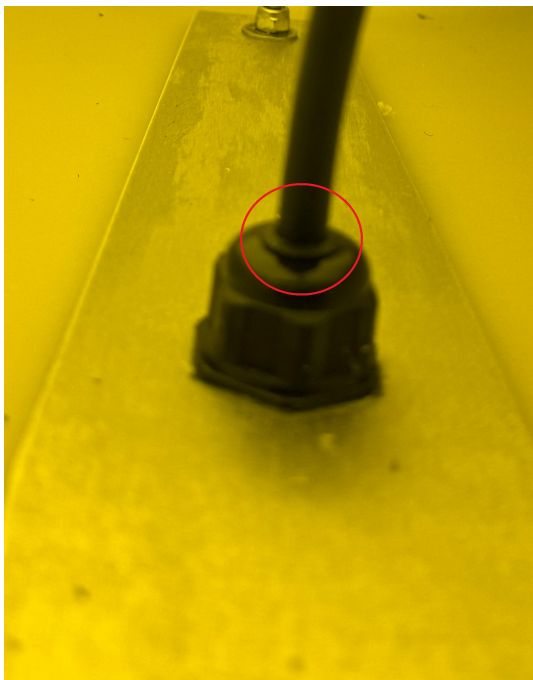
(a) Cable Gland Seal Location
