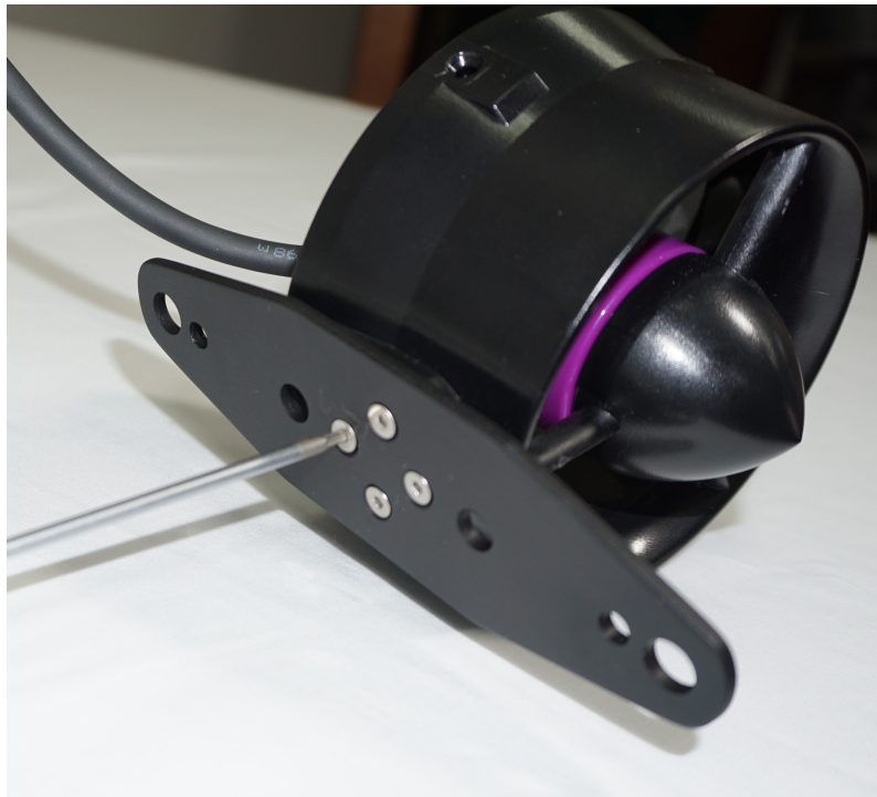
Figure 62: Thruster Adapter Plate Removal
