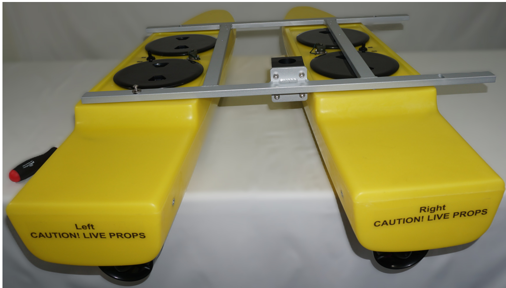
Figure 9: Pontoons Not Spaced Correctly
