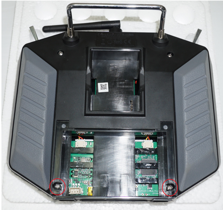
Figure 70: RCU Additional Screw Locations
