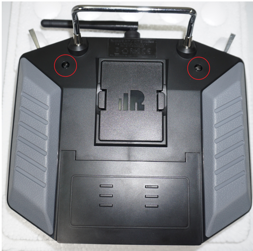
Figure 69: RCU 2x Screw Locations
