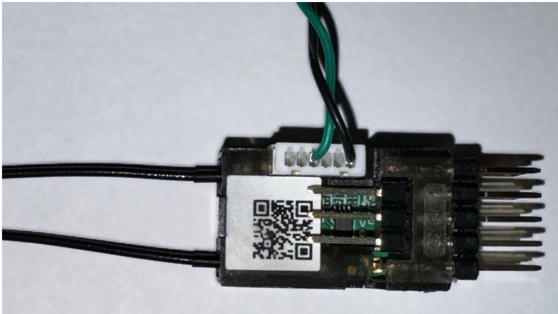
Figure 33: Receiver AIN2 Connection
