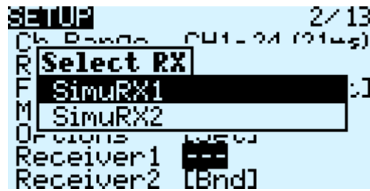
Figure 38: Binding Screen - SimuRX1/2 Is Only Used For Simulation
