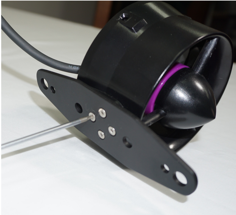
Figure 57: Thruster Adapter Plate Removal
